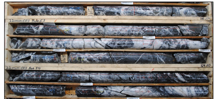
22MM-003 drill core photo depicting high density veining encountered within a 50.2 m intercept of 0.66 g/t Au (drill core length)
