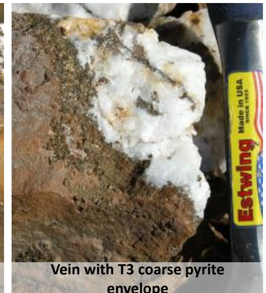
Sheeted veins in discrete T3 carbonate-pyrite alteration
