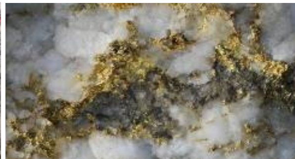
Quartz vein with band of coarse gold and pyrite, Bain (above); Bain vein in historical stope (left)
