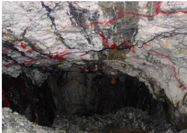
Quartz vein with band of coarse gold and pyrite, Bain (above); Bain vein in historical stope (left)
